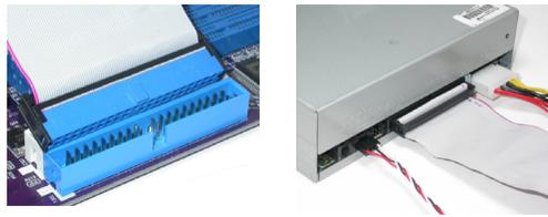
IDE devices enclose jumpers or switches used to set the IDE device as MASTER or SLAVE. Refer to the IDE device user's manual. Installing two IDE devices on one cable, ensure that one device is set to MASTER and the other device is set to SLAVE. The documentation of your IDE device explains how to do this.
